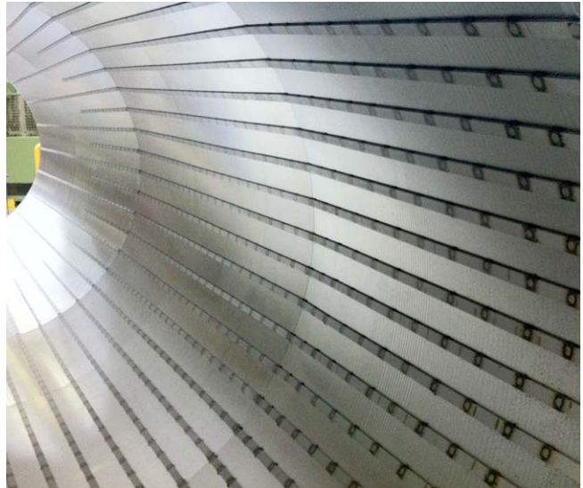
The inside of the bowl is fully protected against abrasive media.
